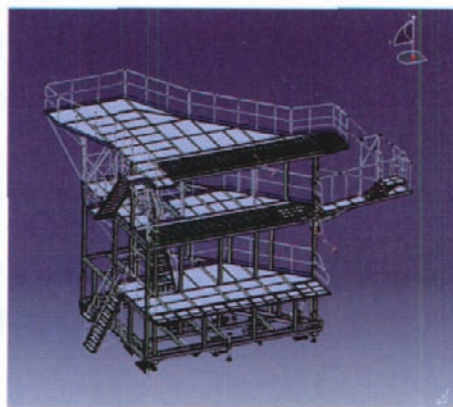
图8 商飞C919平尾装配台(制造中) Fig.8 Aircraft assembly of C919 in COMAC
